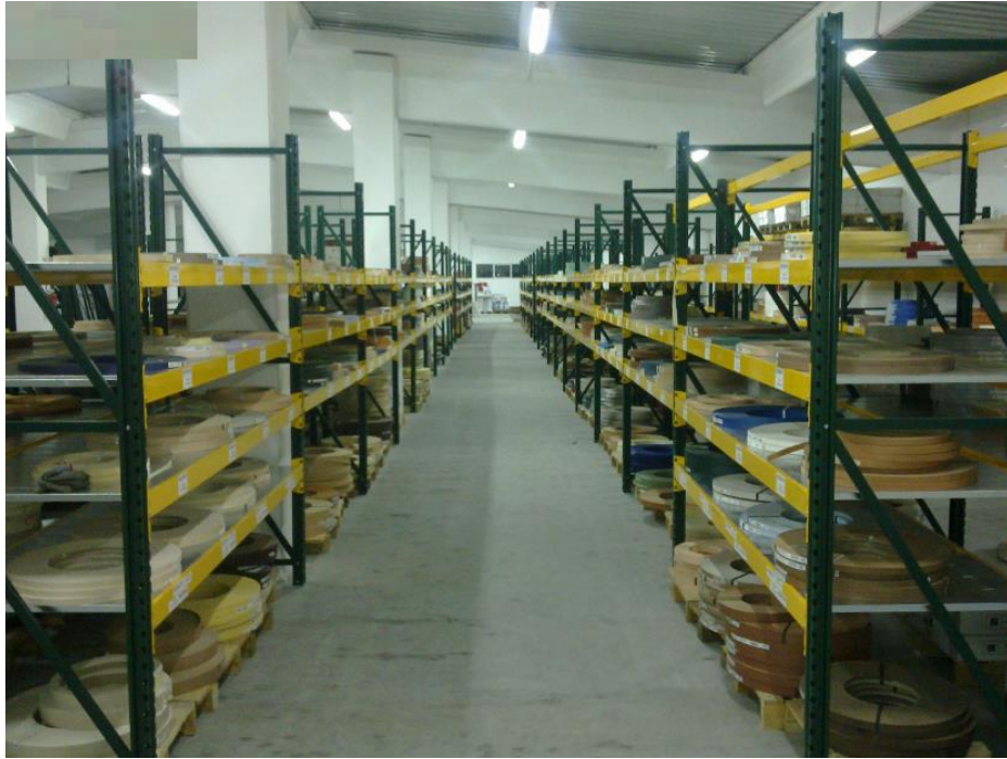
Figure 8: New orientation of rack passages in order to increase flow in the warehouse
