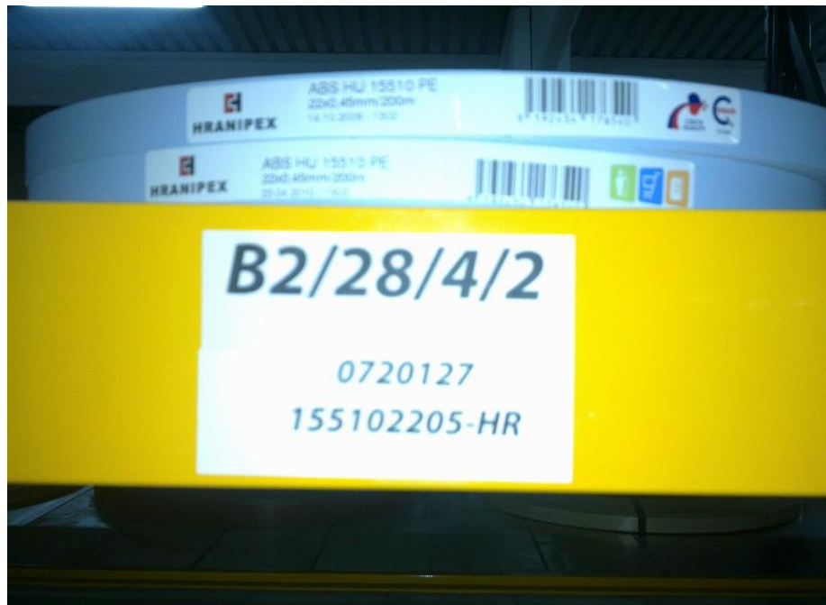
Figure 9: Commissioning location address
